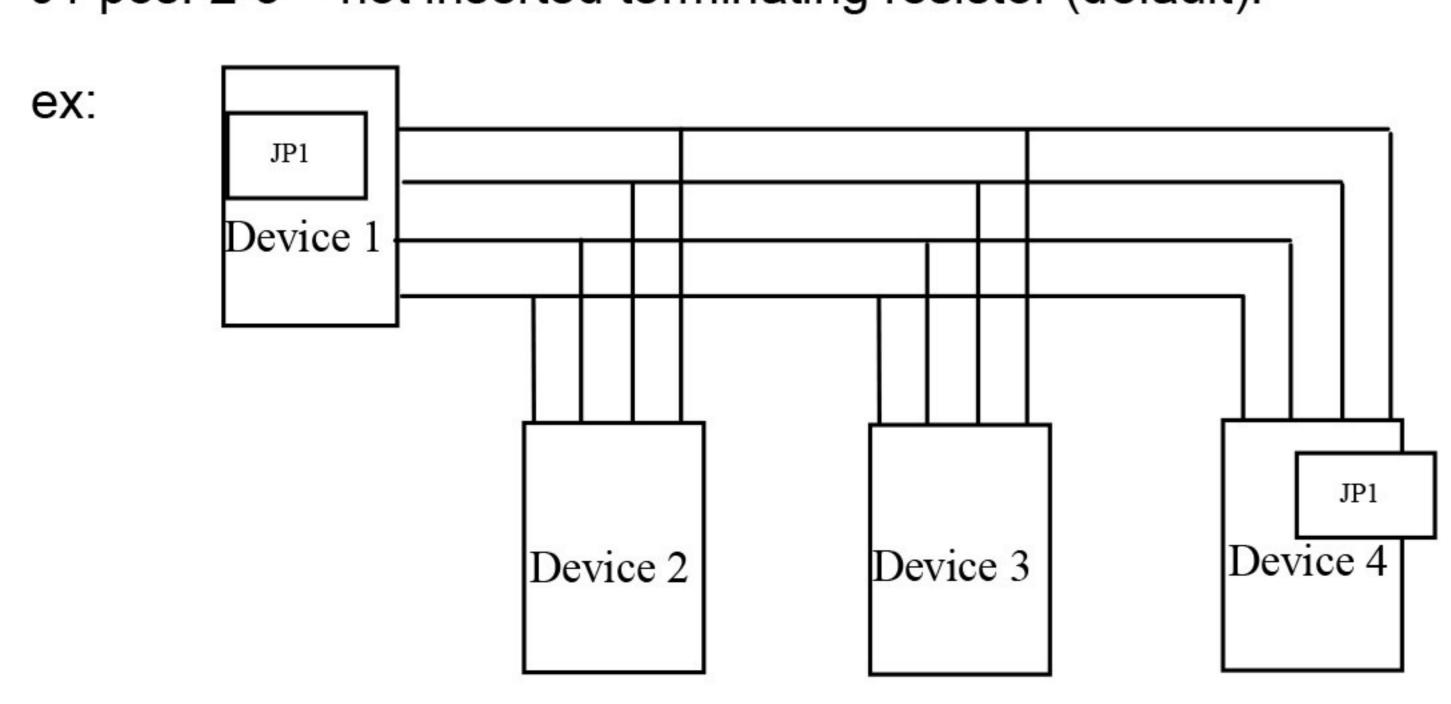
In the example above the jumpers should be placed on devices n. 1 and n. 4, irrespective of the type of device.
