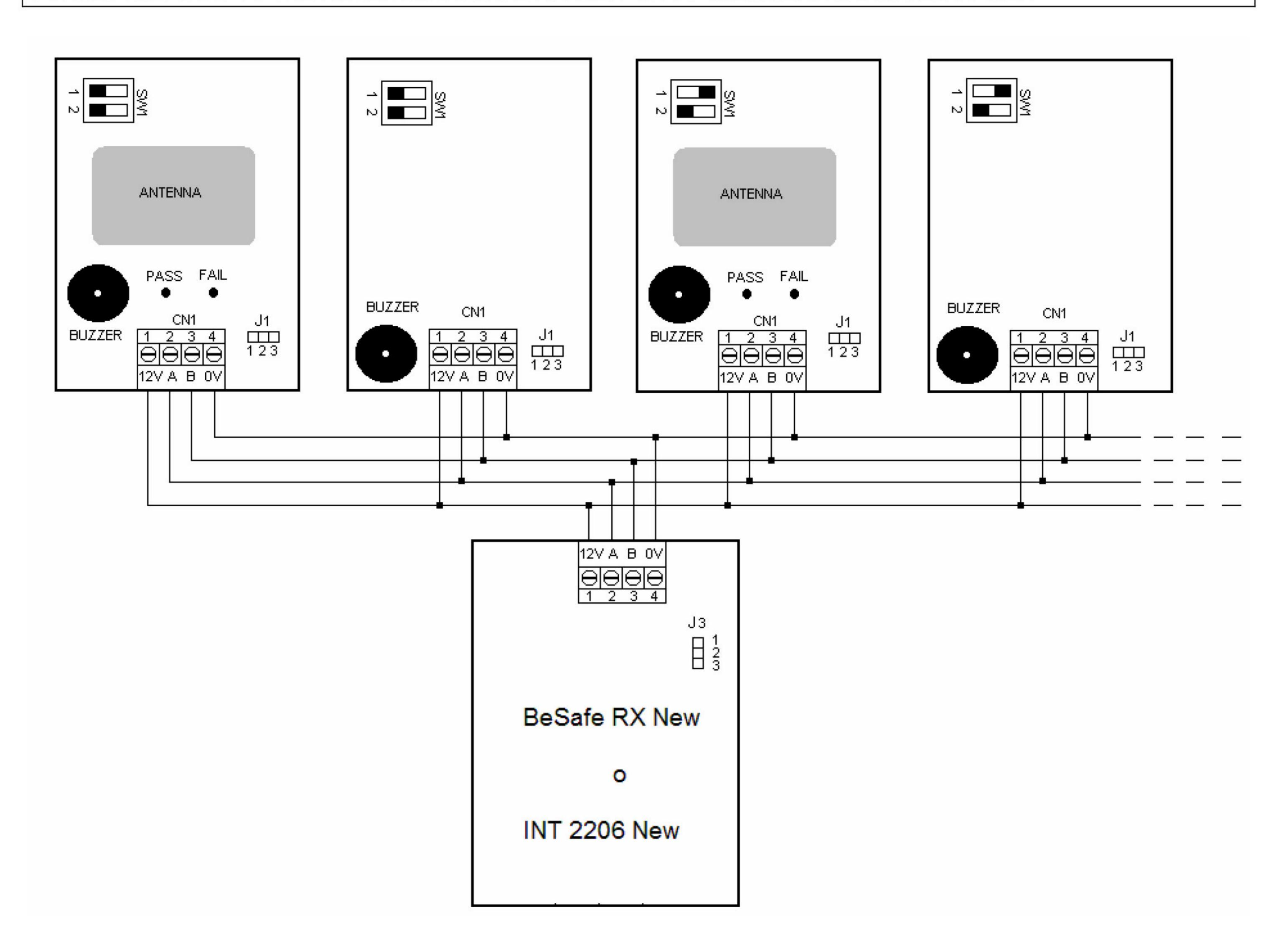
It is possible to connect to every single BeSafe RX New receiver or Interface INT 2206 NEW up to 2 BeSafe Keyboard devices. By dip switch SW1 in advance you must assign to each BeSafe Keyboard its own address:
