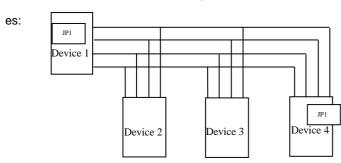
In the example above the jumpers should be placed on devices n. 1 and n. 4, irrespective of the type of device.
