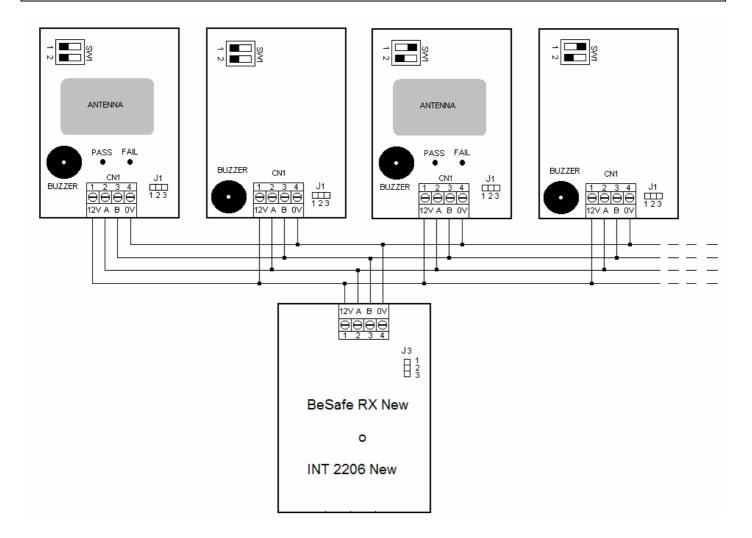
They can be connected to every single receiver BeSafe RX New or Interface INT 2206 New, up to two devices BeSafe Reader New. Using dip switch SW1 it must first be assigned to each of the two BeSafe New Reader its own address:
