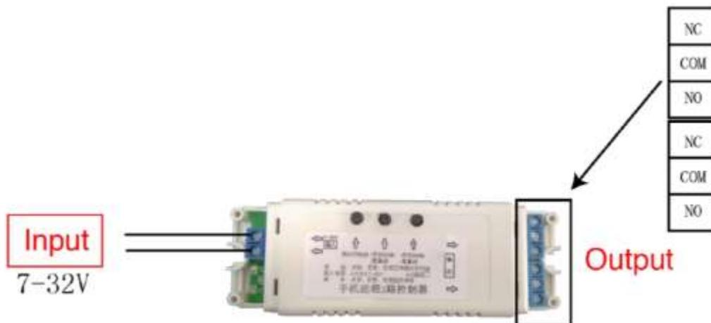
Remark: Input DC/AC 7-32V (Wide Voltage), connection don't need to identify the positive/negative terminal.
